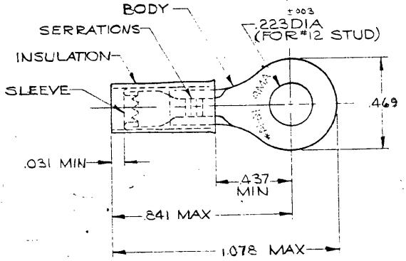
FOR 115 TO 170 WIRE INSULATION DIA.
