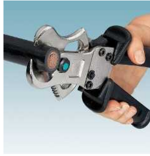
Cable cutter with ratchet function for minimum effort CUTFOX... Page 360
