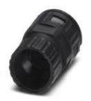
Corrugated pipe adapter, with M32 internal thread, straight, black, IP66, for connecting corrugated pipes to HEAVYCON EVO plastic cable glands or ADVANCE plastic housing.
