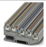
Sensor/actuator terminal block, Connection method: Push-in connection, Cross section: 0.14 mm² - 1.5 mm², AWG: 26 - 14, Width: 3.5 mm, Color: gray, Mounting type: NS 35/7,5, NS 35/15
