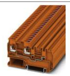
Sensor/actuator terminal block, Connection method: Push-in connection, Cross section: 0.2 mm² - 4 mm², AWG: 24 - 12, Width: 7 mm, Color: orange, Mounting type: NS 35/7,5, NS 35/15
