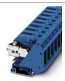
N disconnect terminal block, Special and hybrid connection, Cross section: 0.75 mm² - 35 mm², AWG: 18 - 2, Width: 15 mm, Color: blue, Mounting type: NS 35/7,5, NS 35/15
