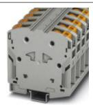
High-current terminal block, nom. voltage: 1500 V, nominal current: 150 A, connection method: Power-Turn connection, number of connections: 2, cross section:10 mm² - 70 mm², AWG: 8 - 2/0, width: 20 mm, color: gray, mounting type: NS 35/15
