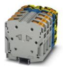
High-current terminal block, Blocked, Connection method: Power-Turn connection, Cross section: 10 mm<sup>2</sup> - 70 mm<sup>2</sup>, AWG: 8 - 2/0, Width: 80 mm, Color: gray/black-yellow, Mounting type: NS 35/15
