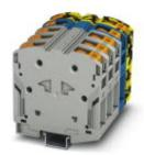
High-current terminal block, Blocked, Connection method: Power-Turn connection, Cross section: 10 mm<sup>2</sup> - 70 mm<sup>2</sup>, AWG: 8 - 2/0, Width: 100 mm, Color: gray/blue/black-yellow, Mounting type: NS 35/15
