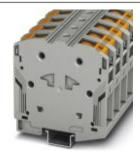
High-current terminal block, Connection method: Power-Turn connection, Cross section: 10 mm<sup>2</sup> - 70 mm<sup>2</sup>, AWG: 8 - 2/0, Width: 20 mm, Color: gray, Mounting type: NS 35/15
