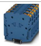
High-current terminal block, nom. voltage: 1500 V, nominal current: 232 A, connection method: Power-Turn connection, number of connections: 2, cross section:25 mm² - 95 mm², AWG: 4 - 4/0, width: 25 mm, color: blue, mounting type: NS 35/15
