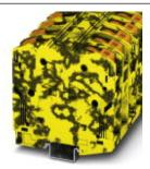
High-current terminal block, Connection method: Push-in connection, Cross section: 25 mm<sup>2</sup> - 95 mm<sup>2</sup>, AWG: 4 - 3/0, Width: 25 mm, Color: black/yellow, Mounting type: NS 35/15
