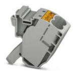
Pick-off terminal block, Connection method: Push-in connection, Cross section: 0.5 mm² - 16 mm², AWG: 20 - 6, Width: 18.5 mm, Height: 34.7 mm, Color: gray, Mounting type: On base element
