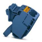
Pick-off terminal block, Connection method: Push-in connection, Cross section: 0.5 mm<sup>2</sup> - 16 mm<sup>2</sup>, AWG: 20 - 6, Width: 18.5 mm, Height: 34.7 mm, Color: blue, Mounting type: On base element
