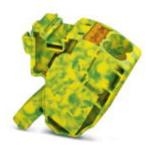
Pick-off terminal block, Connection method: Push-in connection, Cross section: 0.5 mm² - 16 mm², AWG: 20 - 6, Width: 18.5 mm, Height: 34.7 mm, Color: green/yellow, Mounting type: On base element
