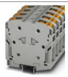
High-current terminal block, Connection method: Push-in connection, Cross section: 25 mm<sup>2</sup> - 95 mm<sup>2</sup>, AWG: 4 - 3/0, Width: 25 mm, Color: gray, Mounting type: NS 35/15
