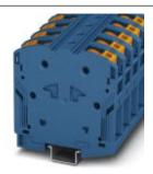
High-current terminal block, Connection method: Push-in connection, Cross section: 25 mm<sup>2</sup> - 95 mm<sup>2</sup>, AWG: 4 - 3/0, Width: 25 mm, Color: blue, Mounting type: NS 35/15
