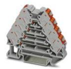
Marshalling panel, Nom. voltage: 250 V, Nominal current: 10 A, Cross section: 0.14 mm² - 2.5 mm², AWG: 12 - 26, Connection type: Push-in connection, Width: 8.3 mm, Length: 64 mm, Color: gray, Assembly: NS 35/7,5, NS 35/15
