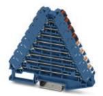
Marshalling panel, Nom. voltage: 250 V, Nominal current: 8 A, Cross section: 0.14 mm² - 2.5 mm², AWG: 14 - 26, Connection type: Push-in connection, Width: 8.3 mm, Length: 100 mm, Color: blue, Assembly: NS 35/7,5, NS 35/15
