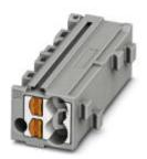
Marshalling patchboard, Nom. voltage: 500 V, Nominal current: 17.5 A, Cross section: 0.14 mm² - 2.5 mm², AWG: 12 - 26, Connection type: Push-in connection, Number of positions: 1, Number of connections: 4, Width: 11 mm, Length: 8.6 mm, Color: gray, Color of connection elements: white, Assembly: for snapping onto a DIN rail adapter, for snapping onto a cover flange
