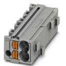
Marshalling patchboard, Nom. voltage: 500 V, Nominal current: 17.5 A, Cross section: 0.14 mm<sup>2</sup> - 2.5 mm<sup>2</sup>, AWG: 12 - 26, Connection type: Push-in connection, Number of positions: 1, Number of connections: 4, Width: 11 mm, Length: 8.6 mm, Color: gray, Color of connection elements: blue, Assembly: for snapping onto a DIN rail adapter, for snapping onto a cover flange
