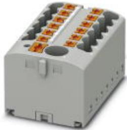
Distribution block, Basic terminal block with supply, nom. voltage: 500 V, nominal current: 24 A, connection method: Push-in connection, Push-in connection, number of connections: 13, cross section: 0.14 mm<sup>2</sup> - 4 mm<sup>2</sup>, AWG: 26 - 12, width: 40.6 mm, height: 21.2 mm, color: gray, mounting type: for snapping onto a DIN rail adapter, Adapter plate
