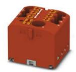
Distribution block, Basic terminal block with supply, nom. voltage: 500 V, nominal current: 24 A, connection method: Push-in connection, Push-in connection, number of connections: 7, cross section:0.14 mm² - 4 mm², AWG: 26 - 12, width: 25.2 mm, height: 21.2 mm, color: red, mounting type: adhesive
