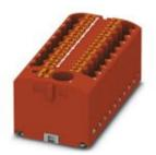
Distribution block, Basic terminal block with supply, nom. voltage: 500 V, nominal current: 24 A, connection method: Push-in connection, Push-in connection, number of connections: 19, cross section:0.14 mm² - 4 mm², AWG: 26 - 12, width: 56 mm, height: 21.2 mm, color: red, mounting type: adhesive
