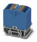
Distribution block, Block with horizontal alignment, nom. voltage: 500 V, nominal current: 24 A, connection method: Push-in connection, number of connections: 6, cross section:0.14 mm<sup>2</sup> - 4 mm<sup>2</sup>, AWG: 26 - 12, width: 15.6 mm, height: 30 mm, color: blue, mounting type: NS 15
