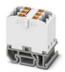
Distribution block, Block with horizontal alignment, nom. voltage: 500 V, nominal current: 24 A, connection method: Push-in connection, number of connections: 6, cross section:0.14 mm² - 4 mm², AWG: 26 - 12, width: 15.6 mm, height: 30 mm, color: white, mounting type: NS 15
