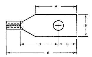
Listed below are A-MP Long Barrel Solistrand Terminals for Bu-Ship Terminal Blocks. See A-MP Instruction Sheet No. 1198 for PIDG and Instruction Sheet No. 1207 for Diamond Grip (DG) Part Numbers.
