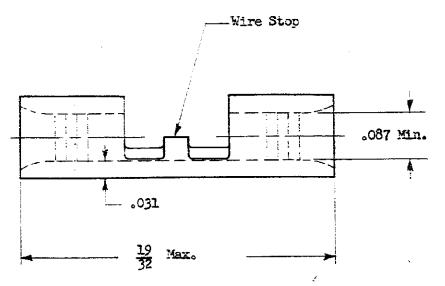
MAX FEATURE LENGTH DOES NOT INCLUDE MANUFACTURING TABS.
