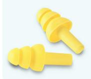
Premolded plugs are made from flexible materials that are preformed to fit the ear. They are generally available with a joining cord to prevent loss. Although the version pictured at the left is a one-sized product, many premolded plugs are sold in two or more sizes and must be **individually sized for each ear**. If after a period of regular wear you've been unable to get used to your earplugs, try another size, type, or brand of hearing protector.
