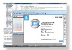
The LonScanner FX Protocol Analyzer is an easy-to-use Windows tool that lets manufacturers, system integrators, and end users observe, analyze, and diagnose the behavior of LonWorks® networks. It provides the advanced productivity features common in data network analyzers, adapted to the unique needs of control networks.
