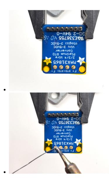
Solder in both pins of each terminal block. You can
