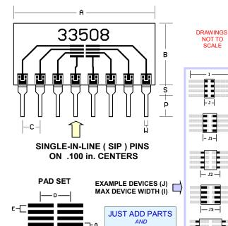
MOUNTING PADS ARE OVERSIZED IN LENGTH TO ACCEPT A WIDER RANGE OF DEVICE WIDTHS AND TOLERANCES AND TO PERMIT HAND SOLDERING. SEE WEBSITE FOR SOLDERING SUGGESTIONS
