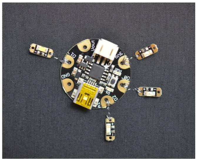
After sewing the positive leads, stitch a line from GND on your microcontroller to connect all sequins' grounds (marked with a -), as illustrated below.
