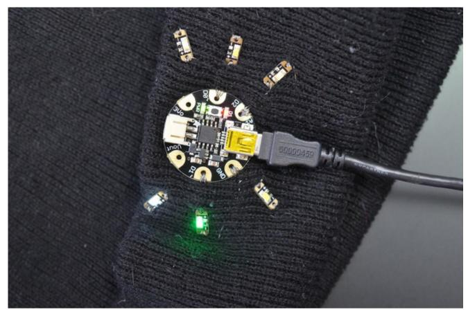
Plug in GEMMA over USB and load the following code into your Adafruit Arduino IDE. If you haven't before, check out our <a href="Introducing GEMMA guide">Introducing GEMMA guide</a> (http://adafru.it/cHH) to get started with the software.
