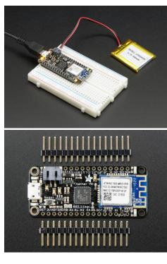
The first option is soldering in plain male headers, this lets you plug in the Feather into a solderless breadboard
