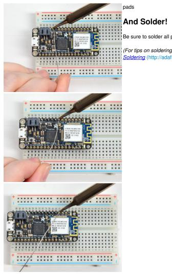
Be sure to solder all pins for reliable electrical contact.
