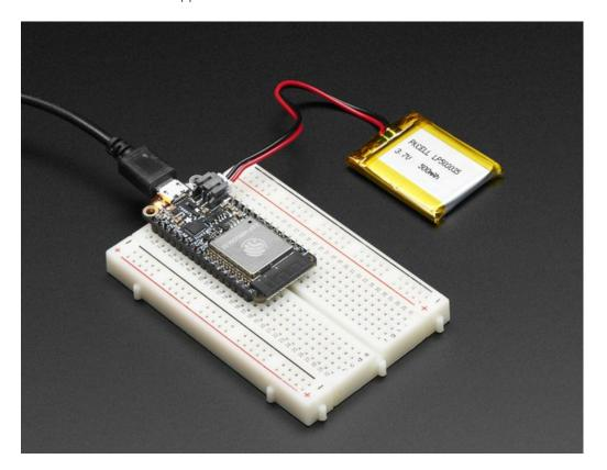
Comes fully assembled and tested, with a USB interface that lets you quickly use it with the Arduino IDE or the low-level ESP32 IDF. We also toss in some header so you can solder it in and plug into a solderless breadboard. Lipoly battery and USB cable not included (but we do have lots of options in the shop if you'd like!)
