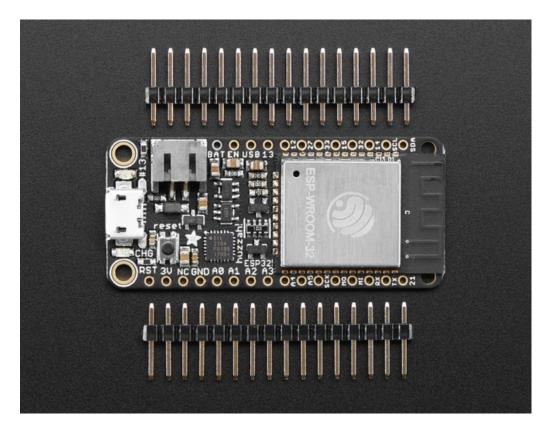
Please note: The ESP32 is still targeted to developers Not all of the peripherals are fully documented with example code, and there are some bugs still being found and fixed. We got all of our Featherwings working under Arduino IDE, so you can expect things like I2C and SPI and analog reads to work. But other elements are still under development. For that reason, we recommend this Feather for makers who have some experience with microcontroller programming, and not as a first dev board.
