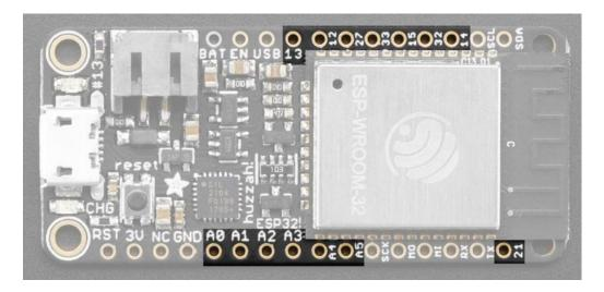
There are tons of GPIO and analog inputs available to you for connecting LEDs, buttons, switches, sensors, etc. Here's the remaining pins available.
