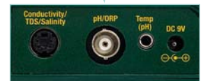
Side inputs for Conductivity Cell, pH/ORP probe, Thermistor probe, and AC Adaptor
