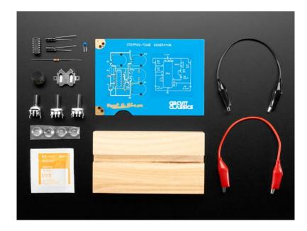
You'll need a couple of additional tools and materials in order to put this kit together: a soldering iron (like this one), and solder. You can use the included wooden stand to hold the board while you solder.
