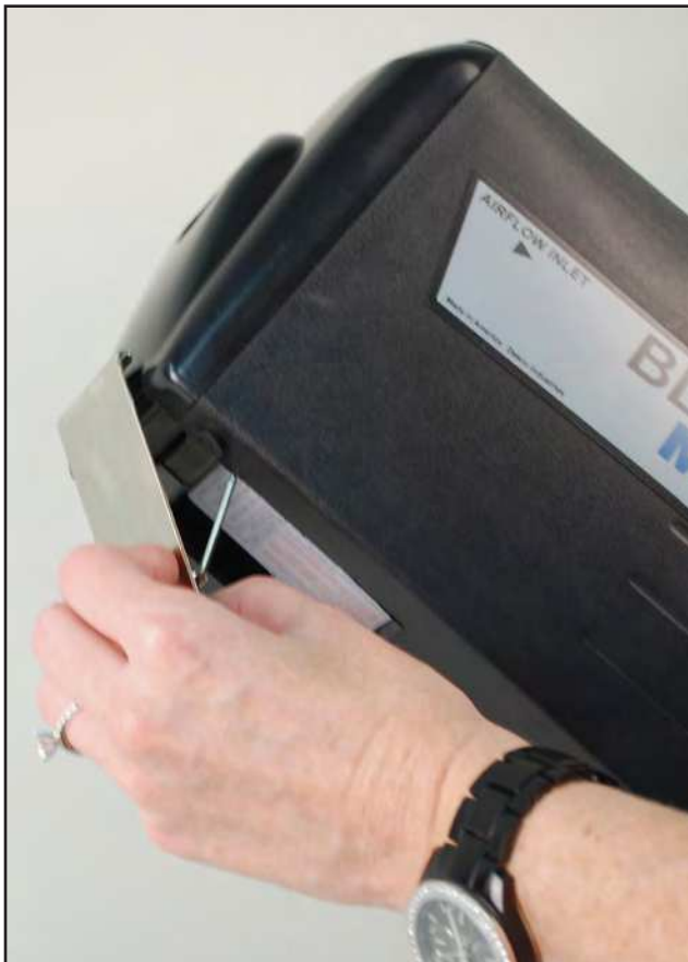
Figure 4: Releasing the Filter
