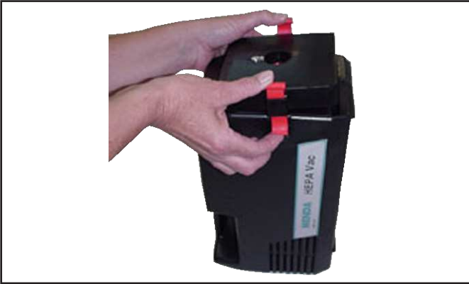
Figure 3: Lifting out the cartridge.
