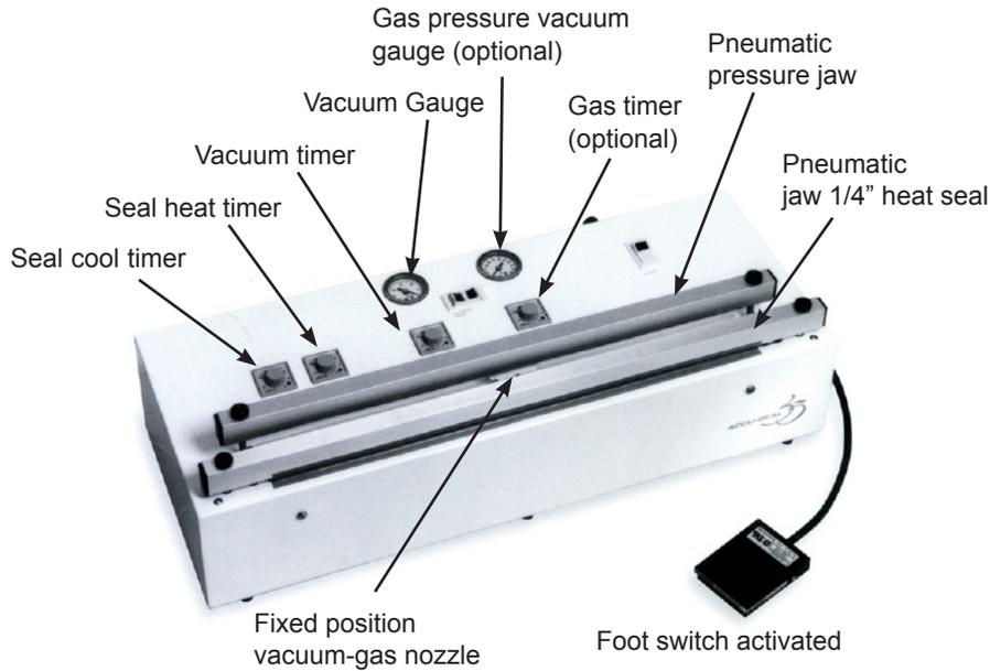
The SCS Vacuum Sealer removes moisture laden air from the interior of moisture barrier bags, and heat seals the bags closed. This is part of the dry packaging process that protects surface mount devices from moisture. For IPC/JEDECJ-STD-033 dry packaging best practice is to include a [moisture barrier bag](#), [desiccant](#), and a [humidity indicator card \(HIC\)](#).
