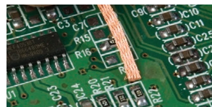
Match braid width to contact area
