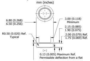
0.06 (0.002) Minimum Ref. (applies to top edge of gasket or edge of crimp, whichever is higher)
