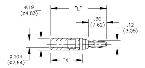
Model 3690 "X" = (11,43mm) 0.45" "L" = (22,61mm) 0.89" Model 4617 "X" = (25,40mm) 1.00" "L" = (36,32mm) 1.43"
