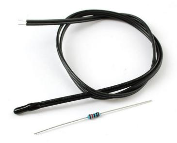
There are two kinds of of thermistors, NTC (negative temperature coefficient) and PTC (positive temperature coefficient). In general, you will see NTC sensors used for temperature measurement. PTC's are often used as resettable fuses - an increase in temperature increases the resistance which means that as more current passes thru them, they heat up and 'choke back' the current, quite handy for protecting circuits!
