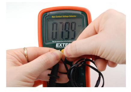
You should read about 10Kohm assuming its room temperature where you're sitting. The resistance of course may be higher or lower depending on the room temperature. For example, its warm here in an un-airconditioned room in the middle of the summer, so we read 8Kohm (30°C - 86°F!)
