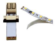
polarity of LEDs as marked with +/- signs along the flex strip, then firmly insert
