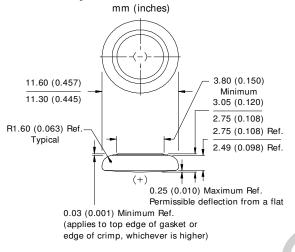
DESIGNED FOR USE ON CONTINUOUS LOW DRAIN (HIGH PULSE ON DEMAND)
