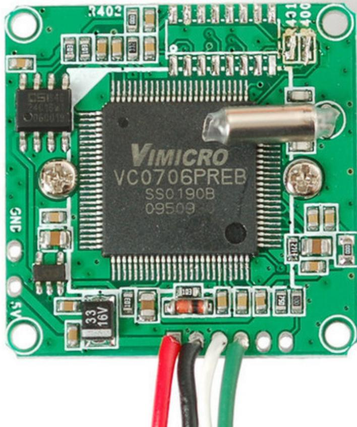
If you'd like to get NTSC video out to connect to a TV or monitor, solder another black wire to the second Ground pin, and a yellow wire to the CVBS pin.
