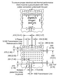
Dimensions are in Inches [Millimeters] 3A412S Mounting Footprint
