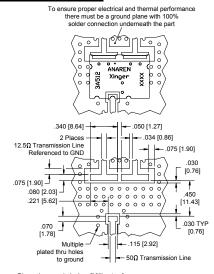
Dimensions are in Inches [Millimeters] 3A512 Rev A Mounting Footprint
