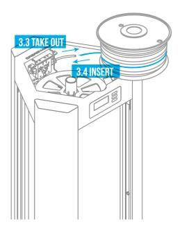
3.4 Insert a new spool of filament into the extruder until it is pulled in automatically;
